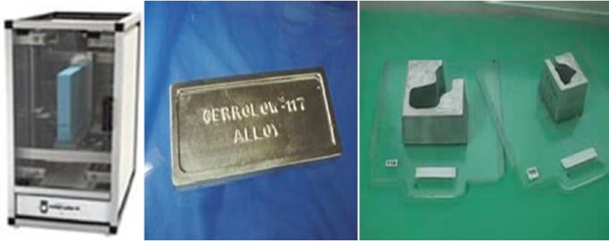
Fig. 1.67 Block cutter, Cerrobend, and focalized blocks
