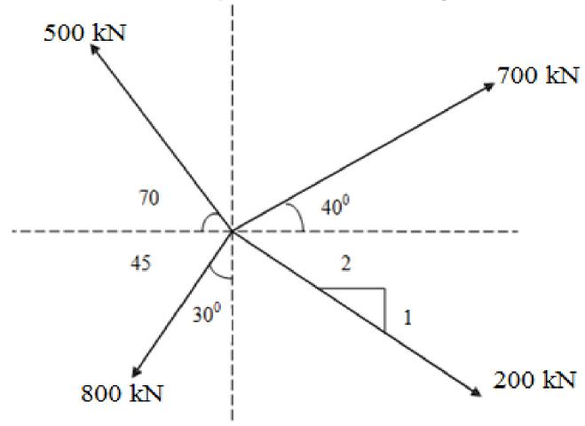
**3.** Determine the resultant of the force system acting on the plate. Also determine the direction of the resultant force as shown in figure given below with respect to AB and AD.
