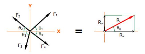
$$R_x = \Sigma F_x \ R_y = \Sigma F_y \ R = \sqrt{{R_x}^2 + {R_y}^2} \ an heta_x = rac{R_y}{R_x}$$
