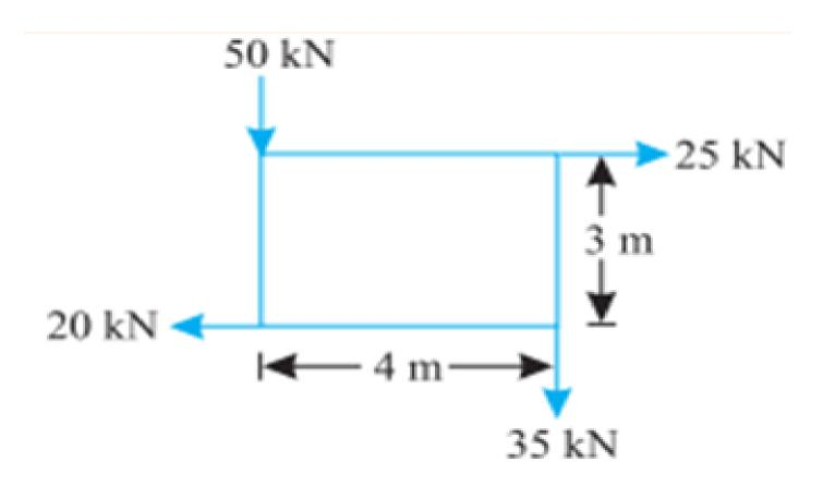
**8.**Locate the amount and position of the resultant of the loads (external forces) acting on the Frank truss shown in figure below.
