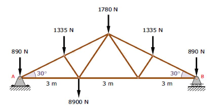
**9.**The Howe roof truss shown in figure below carries the given loads (external forces). The wind loads are perpendicular to the inclined members. Determine the magnitude of the resultant, its inclination with the horizontal and where it intersects with AB.
