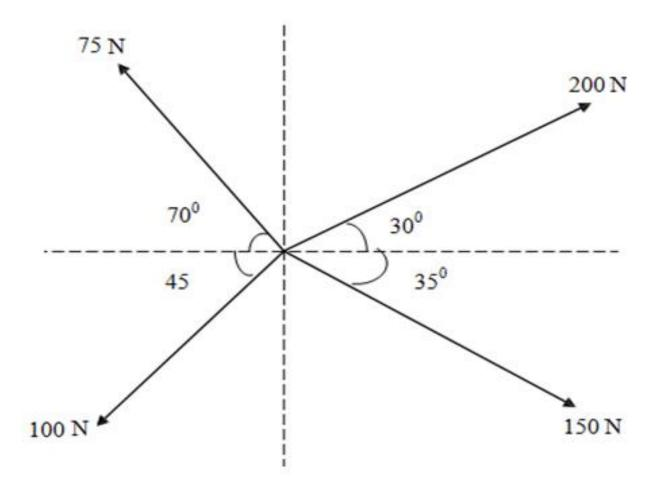
2. Determine the magnitude & direction of resultant of the concurrent force system shown in figure.
