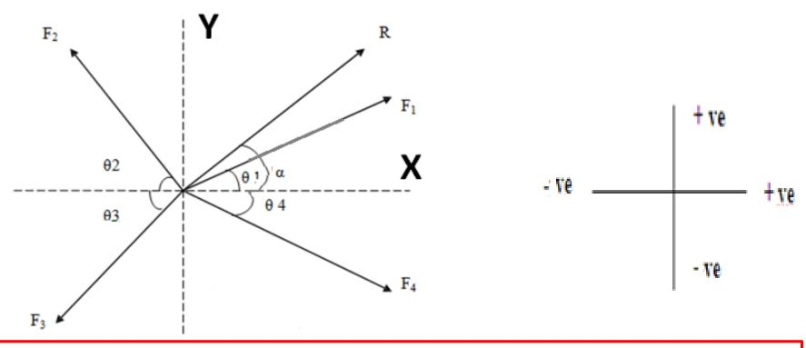
Let  $\Sigma F_x$  be the algebraic sum of component forces in an x-direction  $\Sigma Fx = f_{x1} + f_{x2} + f_{x3} + f_{x4}$
