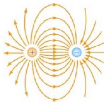
Figure 1.8: Electric field lines for an electric dipole
